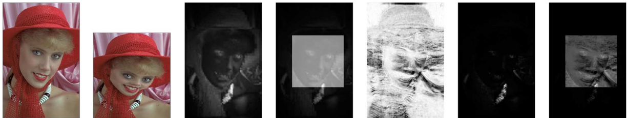
Fig. 5. Left to right: reference image; retargeted image; bottom-up saliency map; overall saliency map (combining bottom-up and top-down saliency maps); SSIM map; point multiplication of SSIM and bottom-up saliency map; point multiplication of SSIM and overall saliency map.
