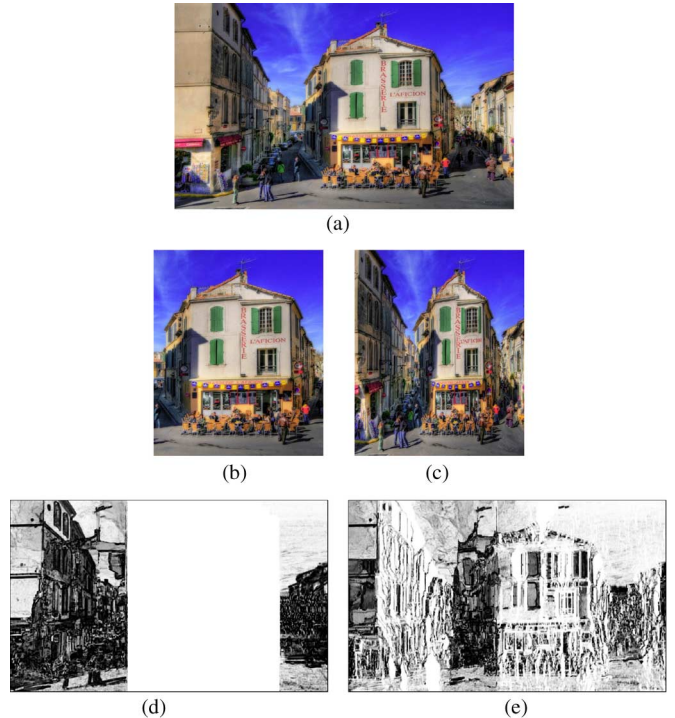
Fig. 2. Examples of SSIM maps. (a) Reference image. (b) Retargeted image by cropping (by 50% of the reference image). (c) Retargeted image by seam carving [4] (by 50% of the reference image). (d) SSIM map of the retargeted image in (b) (the structures of the center region are perfectly preserved, since the SSIM map is generated by directly cropping the center part of the reference image.). (e) SSIM map of the retargeted image in (c). In (d) and (e), brighter pixels indicate higher SSIM values.
